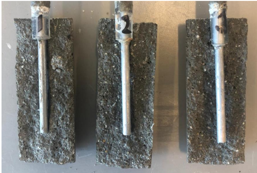
Figure 9: Examination of the steel bars after the potentiostatic test (with admixture).
