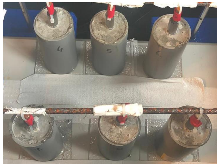
Figure 3: Moulds with the bars in the mortar after 24 hour hardening.
