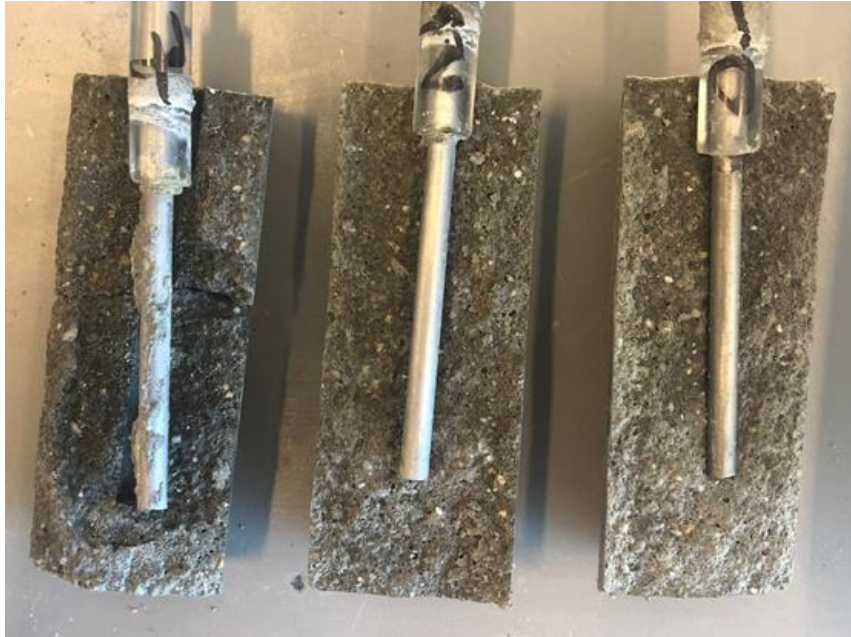
Figure 11: Examination of the steel bars with reference mortar after the potentiostatic test.
