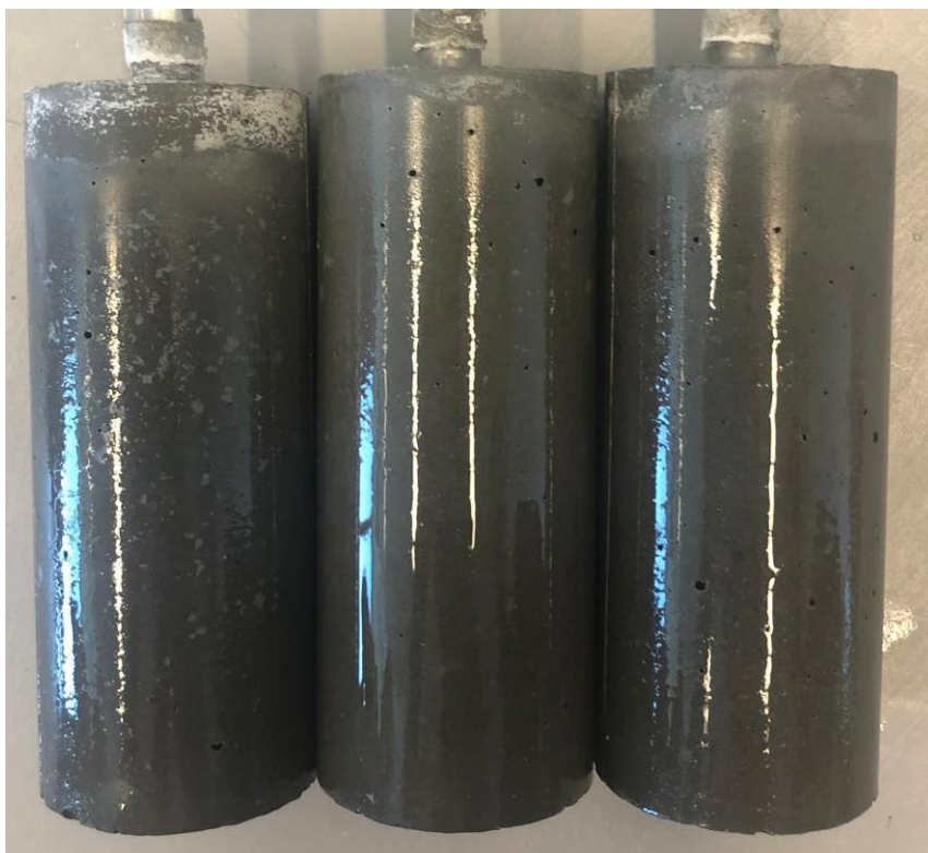
Figure 10: Appearance of sample 4, 5 and 6 with reference mortar after finalizing the tests.
